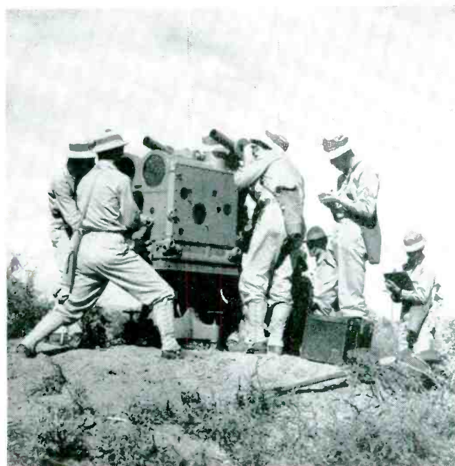
Below: A directional finder used in conjunction with anti-aircraft and heavy field pieces, for directing gunfire.
