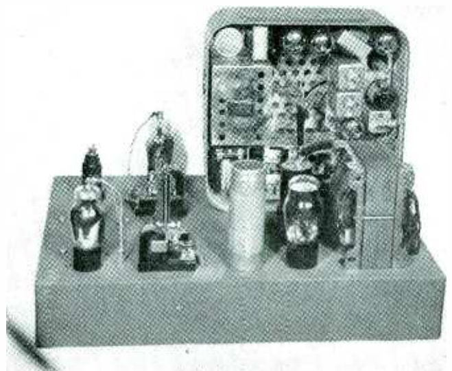
Side and rear chassis views of the alert receiver. Tuner is discarded auto-radio set.
