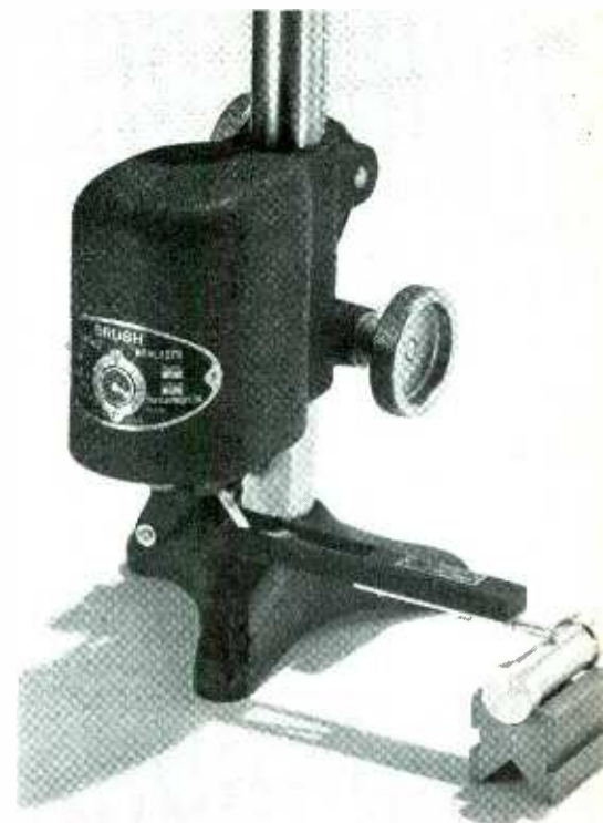
Fig. 3. Pickup arm rotated 90^\circ to facilitate the measuring of intricately shaped surfaces.
