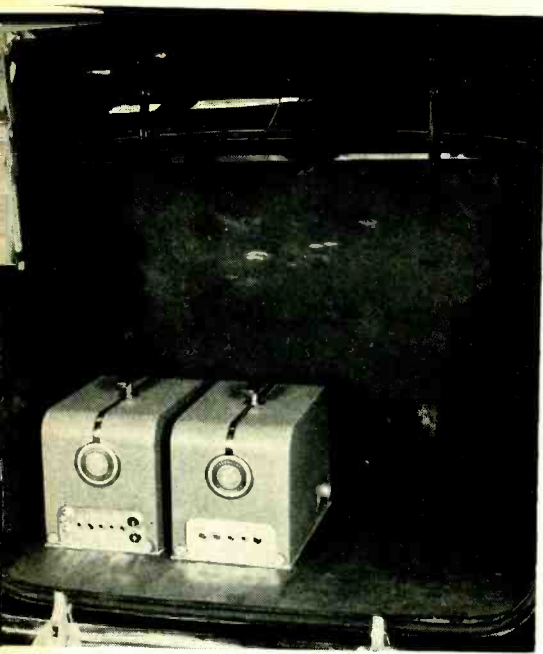
Fig. 7. Side-by-side mounting, and with largest dimension towards the rear, leaves usable prowl-car trunk space.
