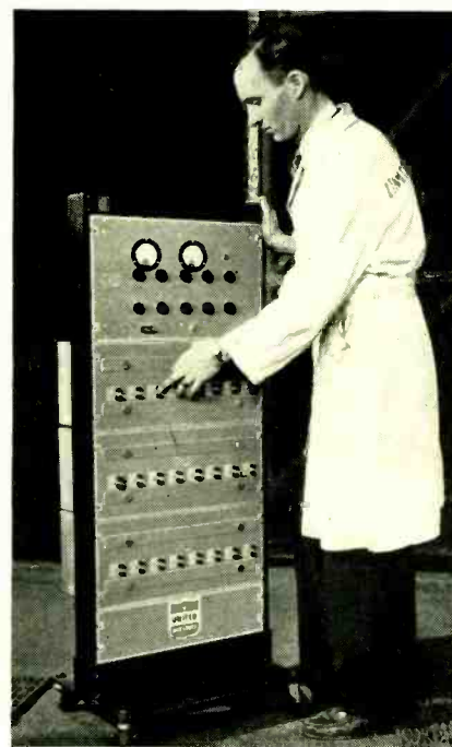
Crystal-controlled push-button signal generator for test and alignment purposes. (Photo courtesy United Airlines).
