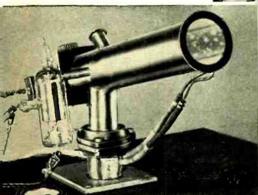
Close observation of the flow of electrons from a heated filament is made possible with this Electron Microscope. This instrument, designed and constructed in the Eimac laboratories, virtually gives a motion picture projection of the electron movement.
