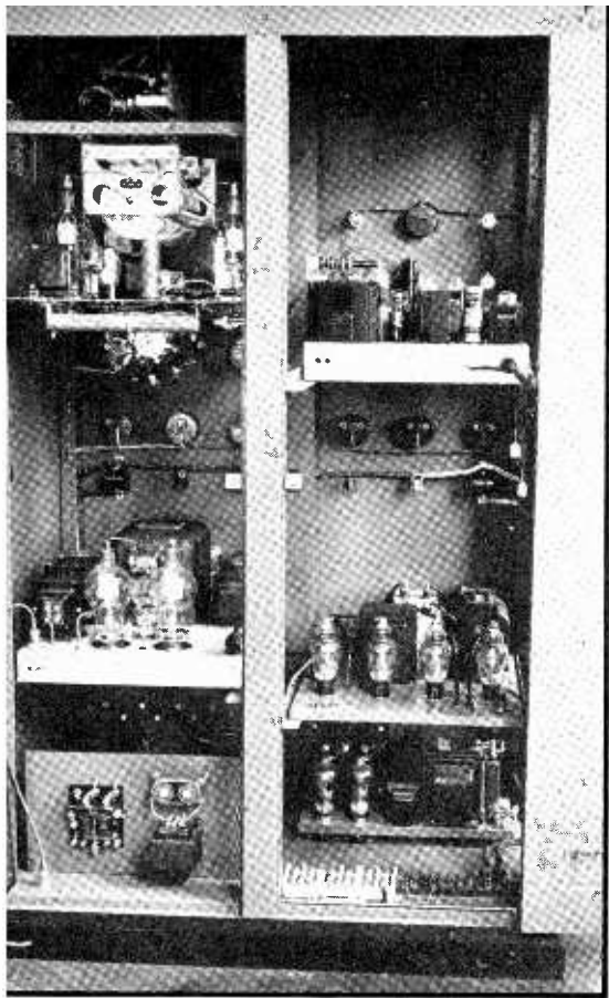
Rear view of the transmitter showing the relative simplicity of construction attained through the use of chassis-type construction.
