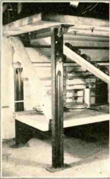
Figure 2. A method of constructing a sturdy and serviceable bench through the use of manufactured pressed-metal legs and horizontal members. Note that additional wood braces are required to stabilize a bench made in this manner.
