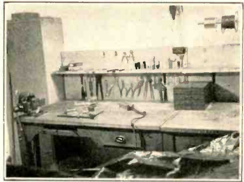
Figure 3. It is always best to have a backboard along the rear of the bench. This board may be made up of about \frac{3}{8} " plywood or of a number of old drawing boards.
