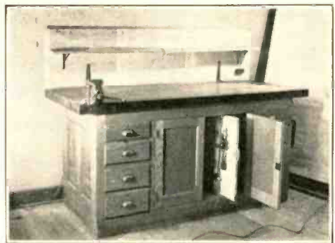
Figure 4. An enclosed-type work bench with three drawing boards along the rear making up the backboard. The shelf along the backboard serves to strengthen it and furnishes additional storage space.
