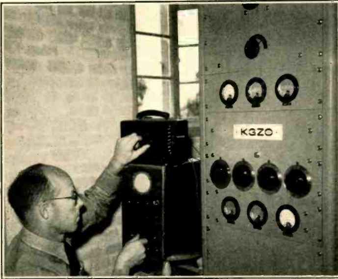
The author setting up the oscilloscope and audio oscillator for running a modulation check on the transmitter.
