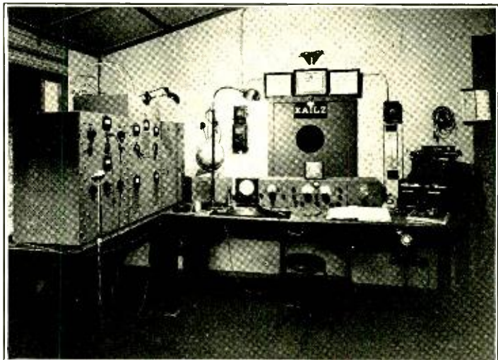
KA1LZ, radiotelephone winner for the Philippines. Left cabinet contains speech equipment and exciter, center cabinet contains 250TH final on top and 250TH modulators beneath, and right hand cabinet houses power supplies.
