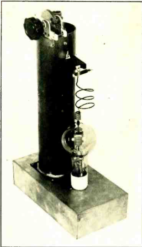
This concentric-line oscillator with a 75T gives good stability and a quite reasonable power output on the 2½-meter band.
