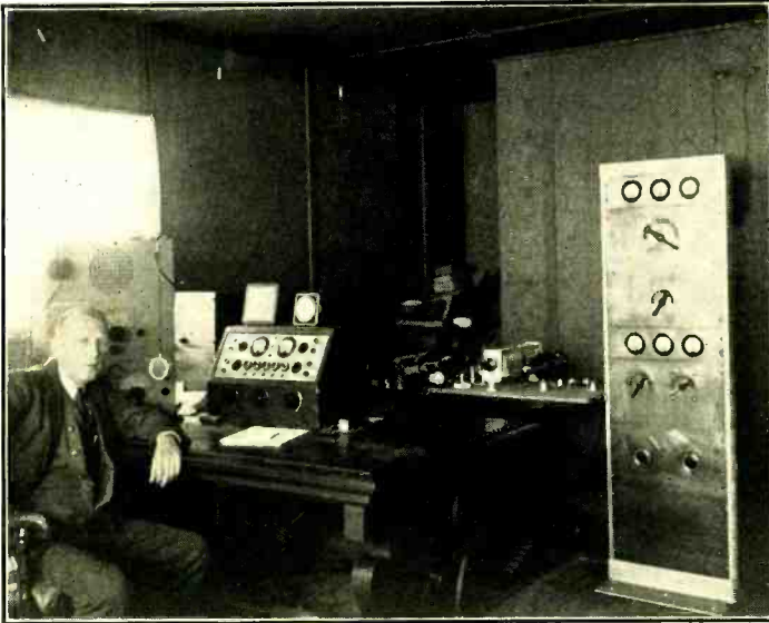
W6OCH — operator, Larry Barton. Transmitter runs a kilowatt into a set of rhombics and phased arrays. Receiver is an RME-69 with DB-20.
