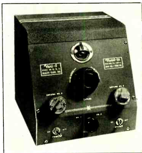
This small cabinet houses the oscillator and its power supply. The large knob at the center of the panel tunes the output circuit to either 80 or 40 meters. Crystals are plugged into the panel, where they are available for quick change or frequency shift.
