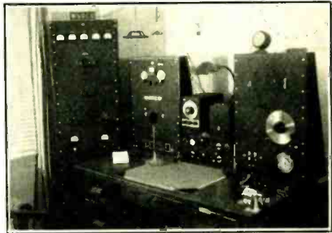
W6RCD was the highest around southern California in the phone division and second high in the district. The rig uses a pair of 100TH's in the final and starts out with an X-EC.
