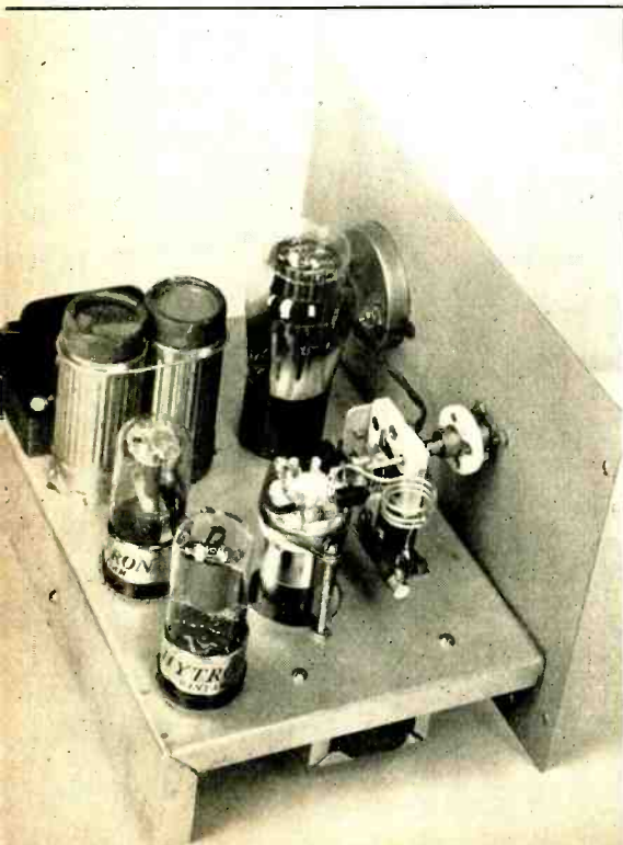
Rear three-quarter view showing layout of components, especially the inverted mounting of the oscillator in the interests of shortened leads.
