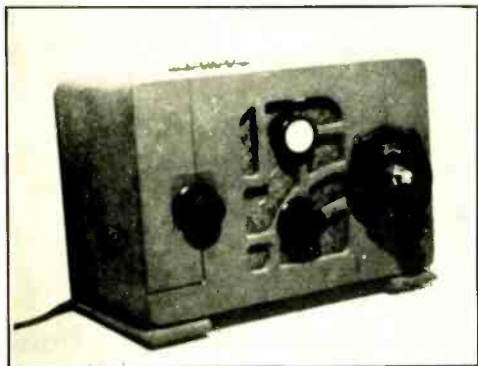
Front view of the revamped midget-set oscilloscope which is used both as a frequency meter and modulation monitor. Note the viewing end of the 913 tube protruding through the former speaker grille.
