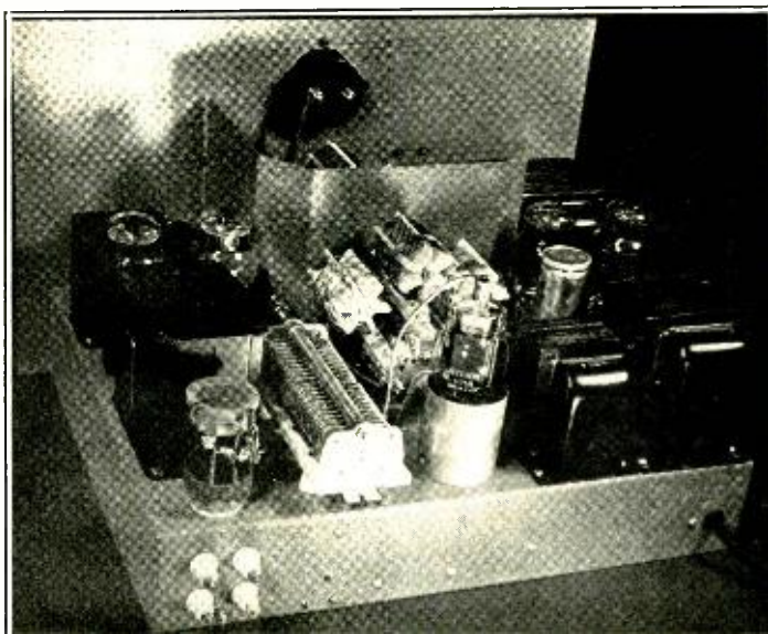
Rear view showing the HY-69 final amplifier, tapped antenna coil, the tank condenser and coil assembly of the final, and the power supplies.
