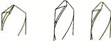
Figure 9 (left). Stoning the edge of a drill so that it presents a flat scraping surface for the drilling of brass. Figure 10 (right). Increasing the angle of clearance of the drill (right hand illustration of the two) so that the point will not wobble through a large hole in sheet material.
