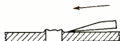
Figure 8. Slicing off with a knife the burr resulting from the drilling of aluminum.
