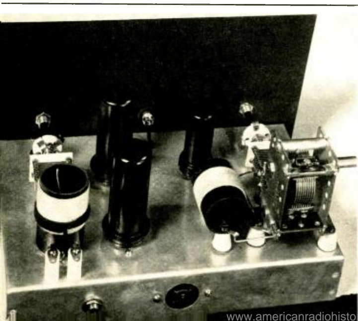
Rear view of the unit. The oscillator components are to the right, the amplifier components to the left. Oscillator components must be firmly supported.
