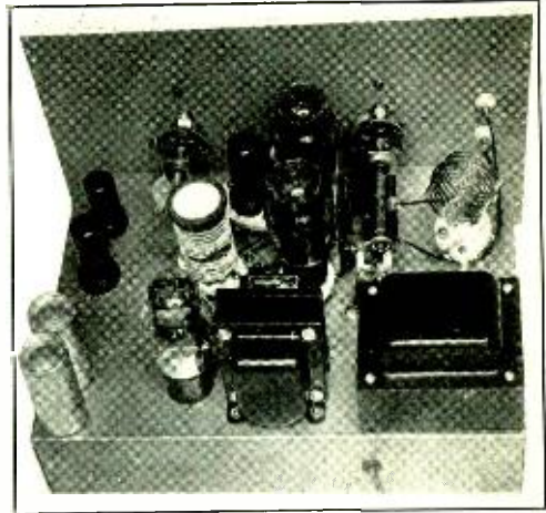
Top view of the chassis of the 6L6G cathode modulated transmitter
