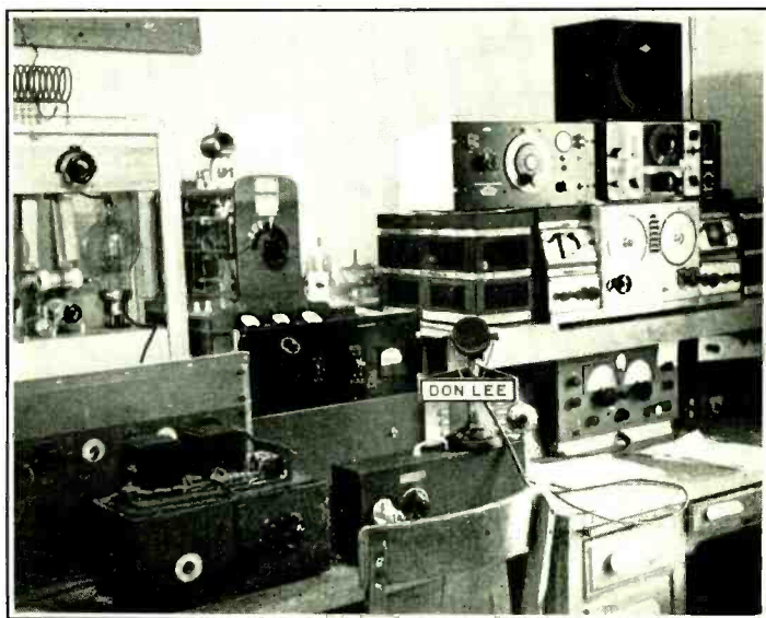
• • • The equipment installation at W6XEJ (W6QD), Los Angeles. The Don Lee speech input and equalizing equipment can be seen on the operating desk to the left in front of the "Corn-Fed Kilowatt."
