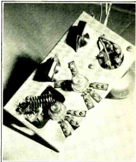
Figure 4. Top view of the diminutive chassis of the three-tube acorn receiver.
