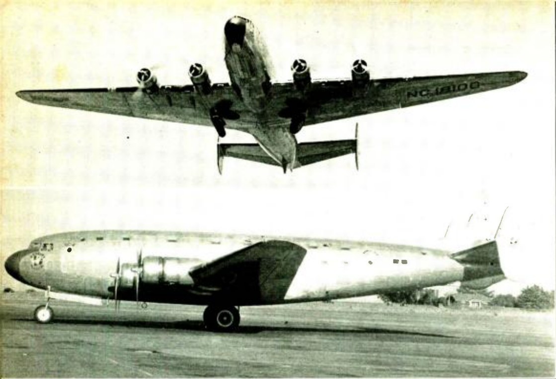
Above, the DC-4 in the air just after the takeoff showing the landing gear being retracted. Below, the ship on the ground showing how it rests on the tricycle landing gear.
