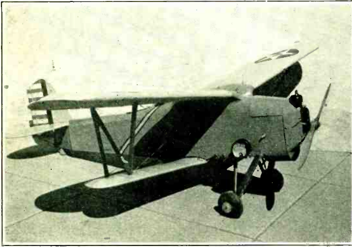
Figure 10. Five foot biplane model which is equipped with radio control. The tuning meter which is removed for flying can be seen just above the landing gear.
