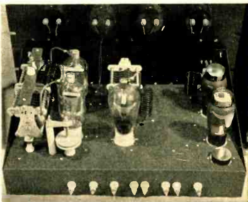
Back view shows layout of the parts in the 10-meter transmitter.
