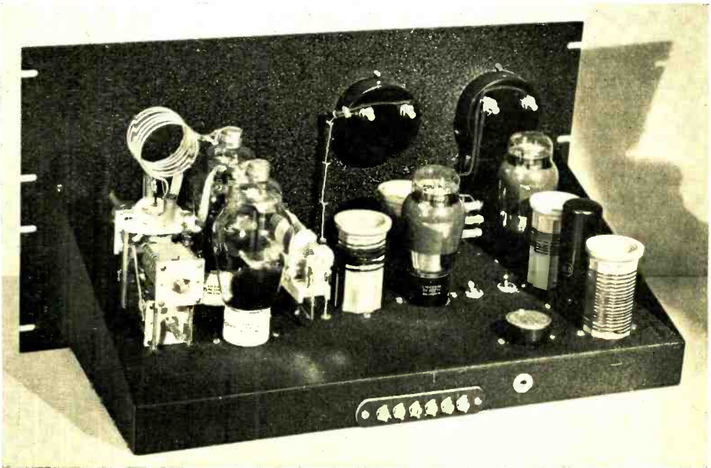
Looking down on the transmitter from the rear. The link line from the 809-grid coil is made just long enough to reach any of the three exciter coils. The 809-tuning condensers are mounted back from the front panel and driven by means of extension shafts.
