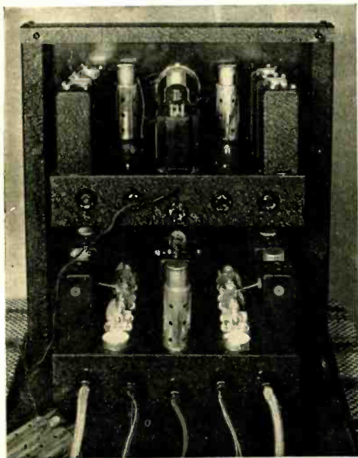
● Back view of the receiver proper. The two i.f. channels, second detectors, and the 6B5 power stage are mounted upon the upper chassis while the two r.f. channels and the h.f. oscillator are on the lower one. The two mixer tubes have been removed from the bottom chassis to show the ganged r.f. tuning condensers. The inter-connecting power and i.f. cables also have been removed for the sake of clearness.
