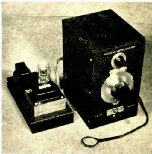
The completed exciter with power supply.
