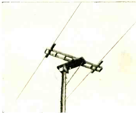
The W5FIY 20-meter installation shows how simply the rotating head can be mounted for rope rotation.
