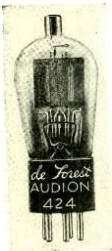
A humless Screen Grid Tube De Forest Audion 424
