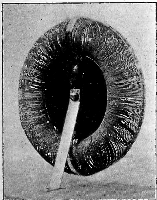
Fig. 6. Rear View of Completed Torusolenoid.
