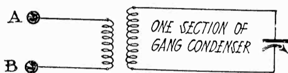
Fig. 3. Connections for Comparing Variable Condensers
