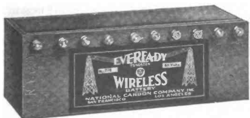
No. 774. The Universal B Battery. One negative and nine positive leads, giving a range of 1½, 3, 4½, 18, 23, 28, 33, 38 and 48 volts.
