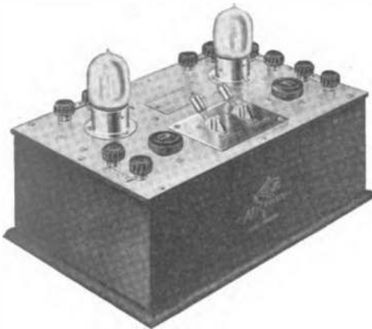
Two-stage power amplifier.
