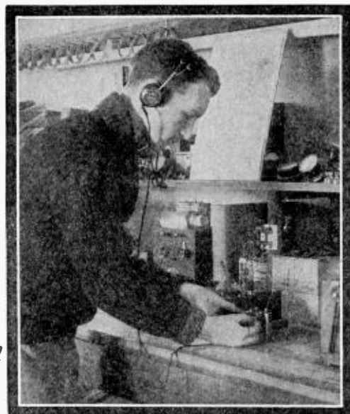
At the left, U. G. Turner, of our laboratory staff, is shown logging stations with the oscillator. At the right, he is testing an audio transformer.
