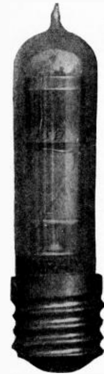
The famous AMRAD "S" tube for rectifying
