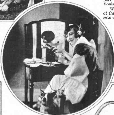
Right — the Kodol P12 two-tube portable receiver, which works a loud-speaker on local and nearby station. Entirely self-contained in a cabinet 5½ inches by 7½ inches by 9 inches and weighs 8 pounds
