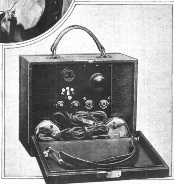
Right — the Kodol P12 two-tube portable receiver, which works a loud-speaker on local and nearby station. Entirely self-contained in a cabinet 5½ inches by 7½ inches by 9 inches and weighs 8 pounds
