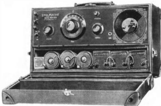
Dropping both lids of the Telmaco reveals the panel, loud-speaker and batteries
