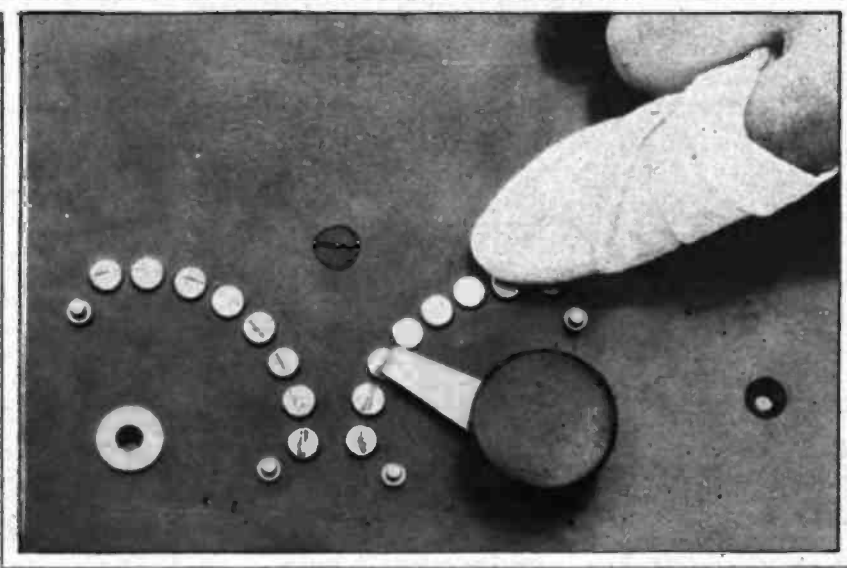
(Fig. 3)—Before sandpapering the socket and tube contacts, take a look underneath and see where the contacting parts are located. Bent springs must be straightened, also
