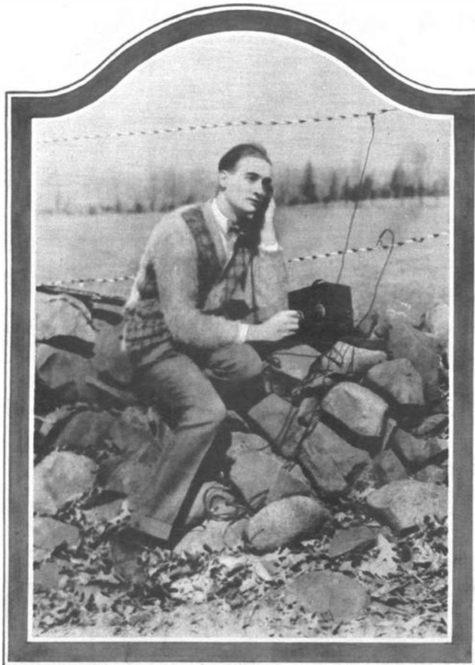
Fig. 1. Mr. Foote finds the two wires of the fence around the cow pasture make a successful aerial and "counterpoise," even though the farmer didn't dream of such a thing when he put them there
