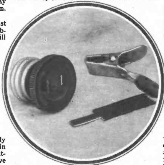
Fig. 7—Above—Here are the necessities for contact to the electric lighting socket. Turn the switch off before you insert the copper strip, also when you change the strip over to the other side of the line
