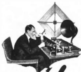
This is H. M. Clarke operating a Super-heterodyne set which he himself built.
