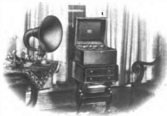
Bristol Single Control Radio Receiving Set, together with Bristol Neuter Audiophone Loud Speaker as used in one of the Fibre Horns.
