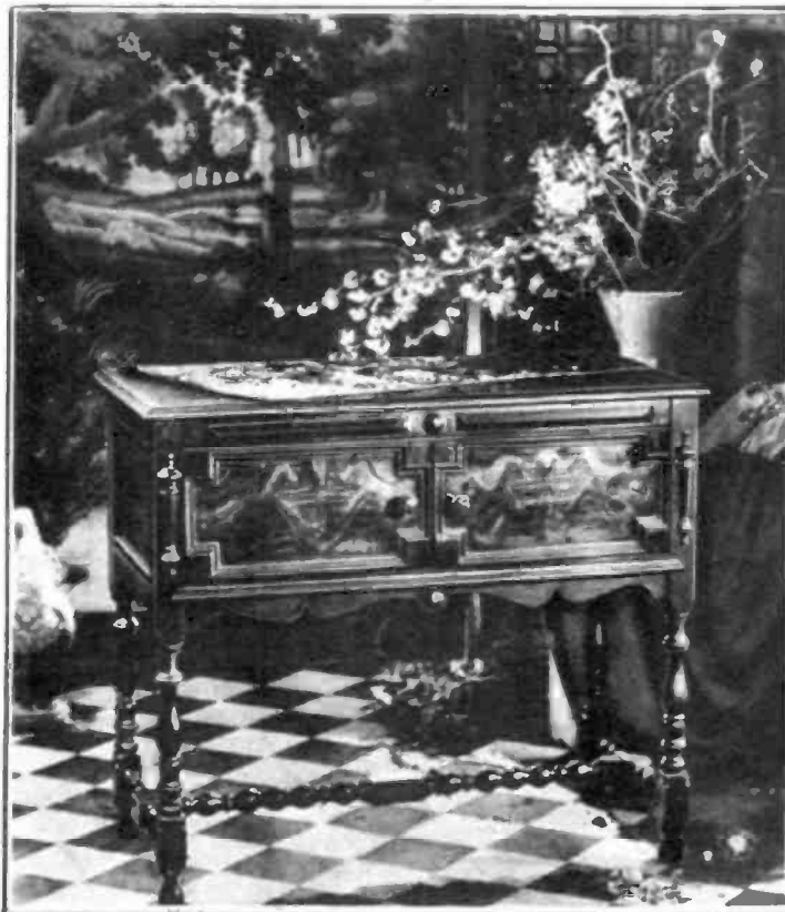
Radio in the home of Arno B. Reincke, Chicago, Ill. All batteries, etc., are contained in the cabinet, and the loud speaker is concealed behind the right-hand door. The set is a Cutting & Washington Console Model of the Teledyne
