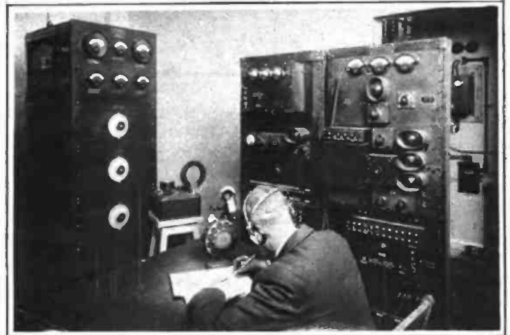
The operating room at Station WEEI. To the left are the combined oscillator and modulator. To the right the control racks, containing monitor circuits, etc. In the right background is the battery and generator room.
