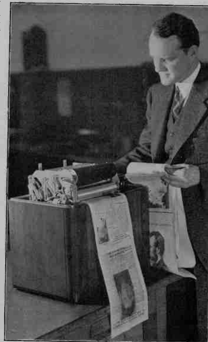
Charles J. Young, RCA Victor research engineer, with the simplified radio facsimile receiver-printer he developed for home use (with the lid-cover removed).
