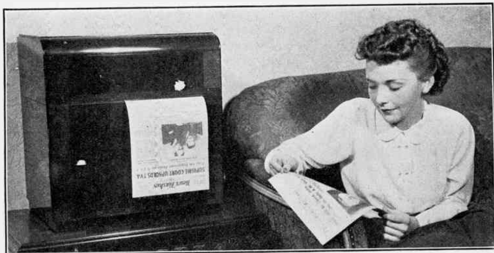
The young lady is reading a facsimile sheet torn from the model that delivers a continuous roll. All the controls are within the cabinet so that they may not get out of adjustment. Page size is 8 1/2 x 12 inches on a continuous roll, printed at the rate of three feet an hour. An automatic time clock arrangement turns the device on and off in accordance with the pre-determined transmission schedule.
