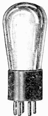
227 detector and RF audio amplifier.
