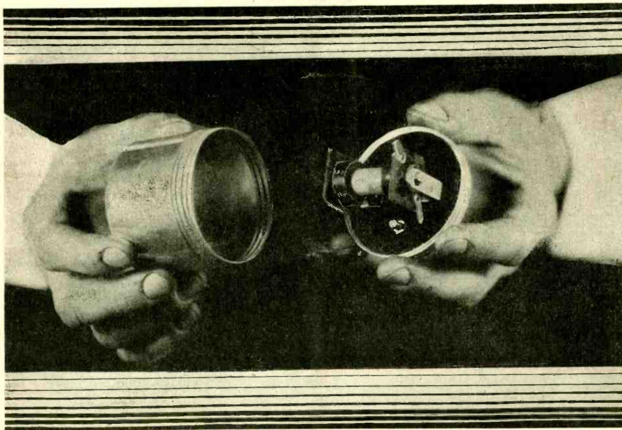
An intermediate transformer may be built in a small aluminum can, with screw cover, adjusting condensers accessible. See pages 5 and 6.
