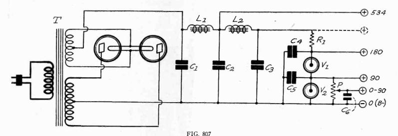
A HIGH VOLTAGE, HEAVY DUTY B POWER SUPPLY UNIT SUITABLE FOR A MODERATE SIZE PUBLIC ADDRESS AMPLIFIER
