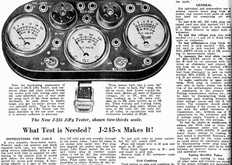
Note the fascinating appearance of the new J-245-X Jiffy Tester, with connector plugs and cable tucked beside the screen grid tube testing cable and the color-identified pair of test leads for using each of the three meters individually. As each meter is double range, you get six-meter service from this splendid outfit. This is the most popular type of Jiffy Tester and the most desirable in the low price range. It is entirely sufficient in accuracy.
