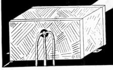
Center-tapped double choke, 125 m.a. rating, 30 henrys in each section. Used for filtering B supply or for a push-pull output impedance, where speaker cords go directly to plates of tubes. Center tap is red. Order Cat. PDC @ \$3.71.
