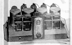
The most sensitive tuned radio frequency tuner so far developed.
