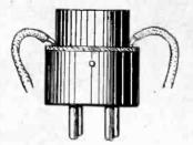
J-24 permits tests of Kellogg and old style Arcturus tubes as filament is on top.
