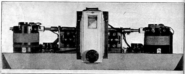
FRONT VIEW, SHOWS THE NATIONAL MODERNIST NUMBERS ARE READ. AT LEFT IS THE ANTENNA STAGE TUNING CIRCUIT. THE COILS
