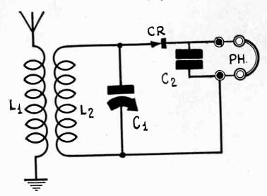
FIG. 19 A CRYSTAL RECEIVER. THE LOW END OF THE SEC-ONDARY MAY BE GROUNDED OR MAY BE LEFT AS
