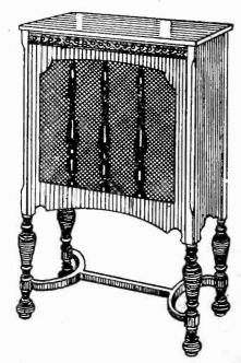
the speaker cabinet is wainut finish. 33" high, 24\(\frac{12}{2}\)" wide, 17\(\frac{1}{2}\)" deep, with carved legs. Golden cloth grille covers front opening. Built inside is No. 59i molded wood born with baffle and No. 203 driving motor unit that stands 258 volts without filtration. Horn and motor removable. Table alone is worth price asked.
