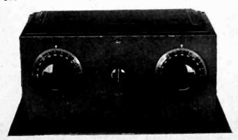
Front view of the FIB Compact. The view is the same for AC or bettery model. For batteries the switch is built in the rheostat. Fur AC a pendant switch is used at rear, in the AC cable.
