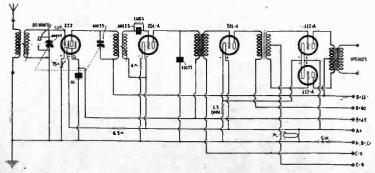
CIRCUIT DIAGRAM OF THE HB 22 FOR USING THE OPEN CONSTRUCTION TUNING UNITS. BOTH THE TUNING CONDENSER ROTOR AND THE PRIMARY IN THE PLATE OF THE RF TUBE ARE RETURNED TO B PLUS, UNDER THIS SYSTEM, BECAUSE THE CONDENSER ROTOR IS INSULATED FROM THE GROUNDED BOTENTIAL BY USE OF A SMALL INSULATED SHAFT. POTENTIAL BY USE OF A SMALL INSULATED SHAFT.
