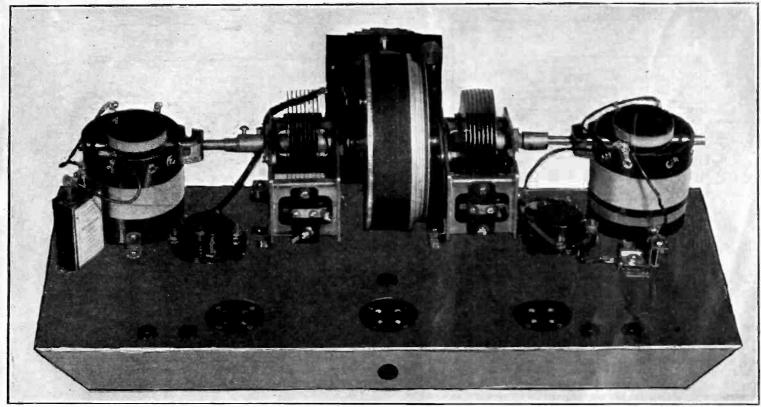
REAR VIEW OF THE TUNER OF THE HB22, SHOWN IN OPEN CONSTRUCTION. EACH COIL-CONDENSER UNIT HAS A SMALL SUBPANEL OF ITS OWN, WITH HOLE DRILLED IN IT TO ACCOMMODATE A SOCKET.
