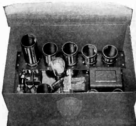
National Thrill Box, 4-tube short wave circuit, 15 to 535 meters, battery-operation of filaments; B supply, either batteries or eliminator.
