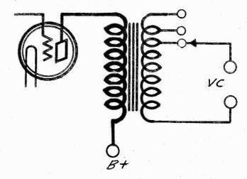
You can use either the whole primary winding in the plate circuit of the power tube or only one-half.
