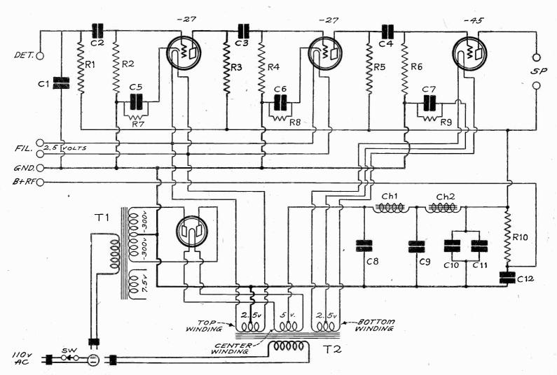
A THREE-STAGE RESISTANCE COUPLED POWER AMPLIFIER FOR OPERATION FROM THE 105-120 VOLT 60 CYCLE AC LINE. THE FILAMENT VOLTAGE FOR HEATER TYPE TUBES OF AN INDEPENDENT RECEIVER IS SUPPLIED, ALSO B VOLTAGE FOR THE RECEIVER. COMPLETE STABILITY IS ASSURED. QUALITY IS EXCELLENT, VOLUME HIGH. NO MOTORBOATING.
