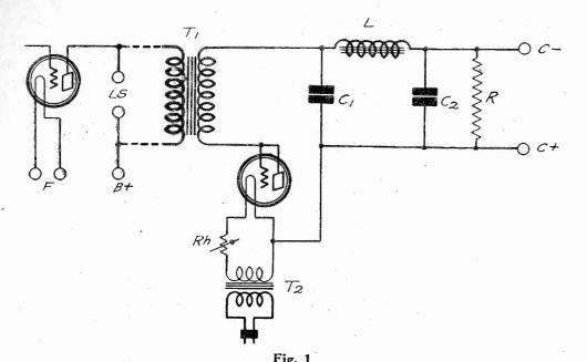
A SIMPLE C BATTERY ELIMINATOR CONNECTED TO THE OUTPUT OF A RECEIVER BY MEANS OF WHICH THE VOLUME OF THE RECEIVER MAY BE CONTROLLED AUTOMATICALLY. THE FILAMENT OF THE RECTIFIER TUBE IS HEATED WITH AC.
