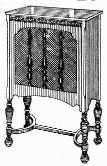
The speaker cabinet is walnut finish, 33" high, 24\\'/2". wide, 17\\'/2". deep, with carved legs. Golden cloth grille covers front opening. Built inside is No. 595 molded wood horn with baffle and No. 203 driving motor unit that stands 250 volts without filtration. Horn and motor removable. Table alone is worth price asked. Remit with order and we pay cartage on Aristocrat Floor Speaker.
