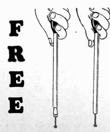
Push out control lever with knob (as at left) and put wrench on nut. Push down on handle only (at right), then turn nut left or right.
