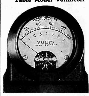
Double range table model voltmeter; scales, 6-74 the scale, for closest observation. The volts and 0-150 volts; made by the Westinghouse Electric & Manufacturing Company. Accurate to 1% plus or minus. Equipped with built-in zero corrector. 34" connecting cable with tip jacks furnished with each meter. Illustration is actual size.
