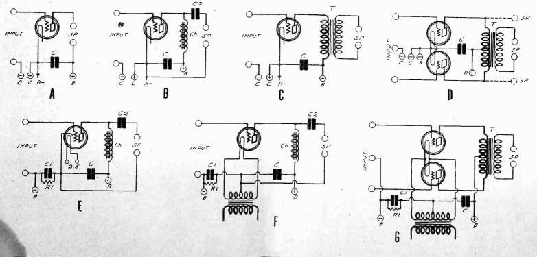
FIG. 9. THE THREE TYPES OF COUPLING BETWEEN THE POWER TUBE AND THE LOUDSPEAKER AS AP-PLIED TO DC AND AC TUBES. A—SPEAKER CONNECTED DIRECTLY IN THE PLATE CIRCUIT; B—THE OUT-PUT FILTER WITH DC TUBE; C—OUTPUT TRANSFORMER WITH DC TUBE; D—PUSH-PULL OUTPUT TRANS-FORMER WITH AC TUBES, AND THE PLATE-TO-PLATE CONNECTION; E—OUTPUT FILTER WITH HEATER TUBE; F—OUTPUT FILTER WITH AC FILAMENT TUBE; G—PUSH-PULL WITH AC FILAMENT TUBES.
