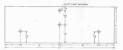
DIMENSIONS FOR THE 7 X 21" FRONT PANEL USED FOR THE PUSH-PULL DIAMOND OF THE AIR. THE VOLUME CONTROL R1 AND SWITCH SW, CONSISTING OF A SINGLE COMPOSITE INSTRUMENT, ARE MOUNTED AT LEFT. THE TUNING CONDENSER IS AT CENTER, 3½" UP. THE PILOT LIGHT, IF USED, IS ABOVE THE CONDENSER. AT RIGHT THE THREE CIRCUIT TUNER IS MOUNTED UPSIDE DOWN, THAT IS, WITH TICKLER COIL TOWARD THE SUBPANEL. THREE HOLES EQUIDISTANT AT BOTTOM MAY BE USED FOR ANCHORAGE TO THE SUBPANEL.
