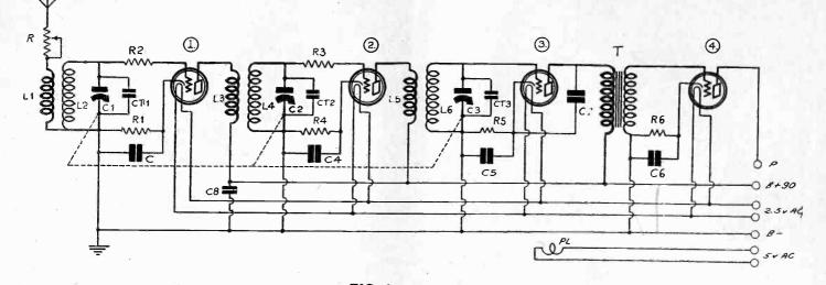
FIG. 1 RECEIVERS CONTAINING HEATER TYPE TUBES CAN BEST BE CONTROLLED AS TO SENSITIVITY AND VOLUME BY MEANS OF VARIABLE GRID BIAS RESISTORS, PLACED IN THE POSITIONS R1 AND R4. THIS IS A LITTLE BETTER THAN THE AERIAL RESISTOR METHOD SHOWN AS R.
