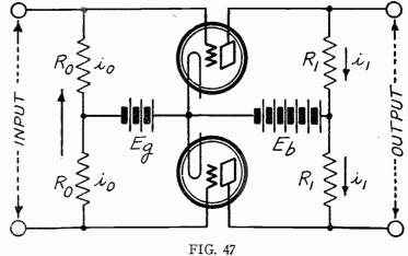
A RESISTANCE COUPLED CIRCUIT FOR ILLUSTRAT-ING PUSH-PULL ACTION.
