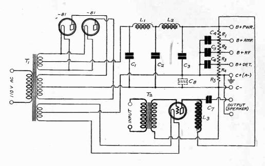
THE bleeder current is that current which flows independent of any plate current drawn by the tubes of a receiver. Thus any resistor across a potential difference will draw current, and this bleeder current exists whether the B supply consists of batteries or an eliminator. However, a bleeder across a battery is a sheer waste and useless. How about a bleeder across an AC B eliminator. B eliminator
