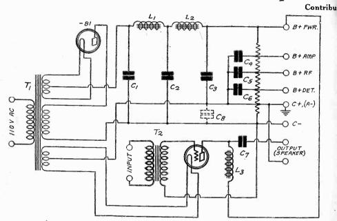
A HALF-WAVE RECTIFIER TUBE IS INACTIVE FOR EACH ALTERNATION (HALF-WAVE RECTIFIER FORE IS INACTIVE FOR EACH ALTERNATION, IT IS (HALF CYCLE) AND ACTIVE DURING THE OTHER ALTERNATION, IT IS ACTIVE WHENEVER THE PLATE IS POSITIVE IN RESPECT TO THE FILA MENT, WHEN THE VOLTAGES ARE VIEWED IN VACUOUS SPACE. IN EXTERNAL PERFORMANCE THE PLATE IS ALWAYS NEGATIVE IN RESPECT TO THE FILAMENT. A SINGLE-SIDED AUDIO OUTPUT IS SHOWN
