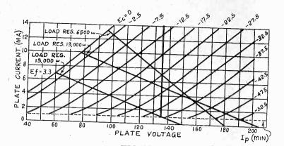
FIG. 71 A FAMILY OF PLATE VOLTAGE, PLATE CURRENT CURVES FOR THE 220 LOW POWER OUTPUT TUBE, WITH THREE LOAD LINES, ONE FOR A RESISTANCE EQUAL TO THE PLATE RESISTANCE AND TWO FOR A RESISTANCE TWICE THE PLATE RESISTANCE.
