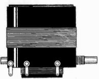
Cat. No. BT5B-\$2.59 FOR .0005 MFD. CONDENSERS Bernard Tuner for working out of a screen grid tube, consists of a rotary coll in series with a fixed col, the two constituting a tuned primary, for tuning the combined rotary and fixed windings to exceed the broadcast band of wavelengths. The condenser shaft and ro-tary coll shaft are physically coupled so one motion turns both. Develops the highest pos-sible amplification from the screen grid tube. Cat. BT3A for .00035 mfd.......\$2.55
