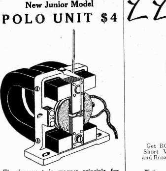
The famous twin magnet principle for double sensitivity, large magnets for great flux, permanently adjusted armature, all are in the new junior model Polo Unit. Weight, 234 lbs. Stands 150 volts unfil-tered. Stands up to 250 push-pull filtered. Works any output tube power or other-Works any output tube, power or other-wise. Supplied with 10-ft. cord. Order unit now. Five-day money-back guarantee.
