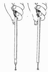
Push out control lever with knob (as at left) and put wrench on nut. Push down on handle only (at right), then turn nut left or right.
