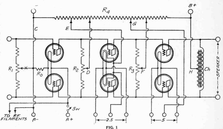
A THREE-STAGE RESISTANCE COUPLED AMPLIFIER SO DESIGNED THAT THERE IS NO HUM IN THE OUTPUT.
