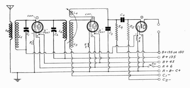
IS ANY ENERGY DELIVERED BY TUBE 1 to TUBE 2? IS ANY ENERGY DELIVERED BY THE DETECTOR TO THE THIRD TUBE IN THIS CIRCUIT? SEE ARTICLE ON THIS PAGE FOR ANSWERS.
