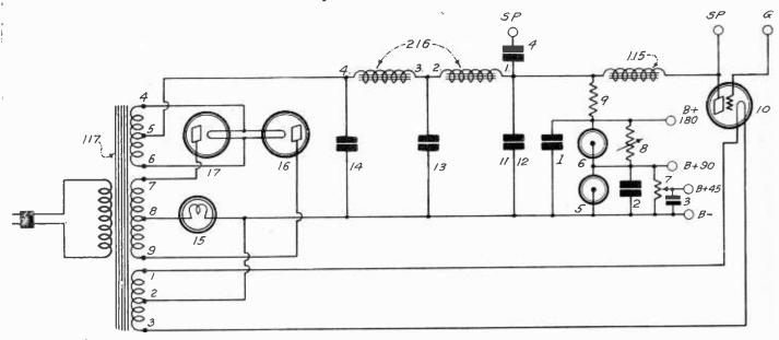
THE CIRCUIT DIAGRAM OF THE VICTOREEN POWER SUPPLY UNIT AND POWER AMPLIFIER.
