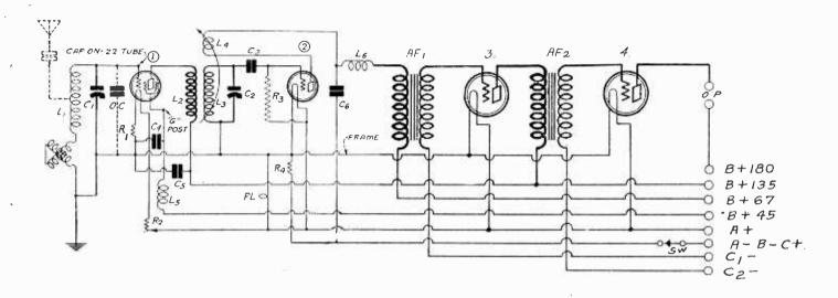
DOES A COUPLING TRANSFORMER IN A CORRECTLY DESIGNED RECEIVER DELIVER POWER OR POTENTIAL TO THE GRID OF THE FOLLOWING TUBE? DOES THE LAST TUBE IN THE RECEIVER DELIVER POWER TO THE LOUDSPEAKER OR MERELY POTENTIAL? SEE ARTICLE HEREWITH FOR ANSWERS.
