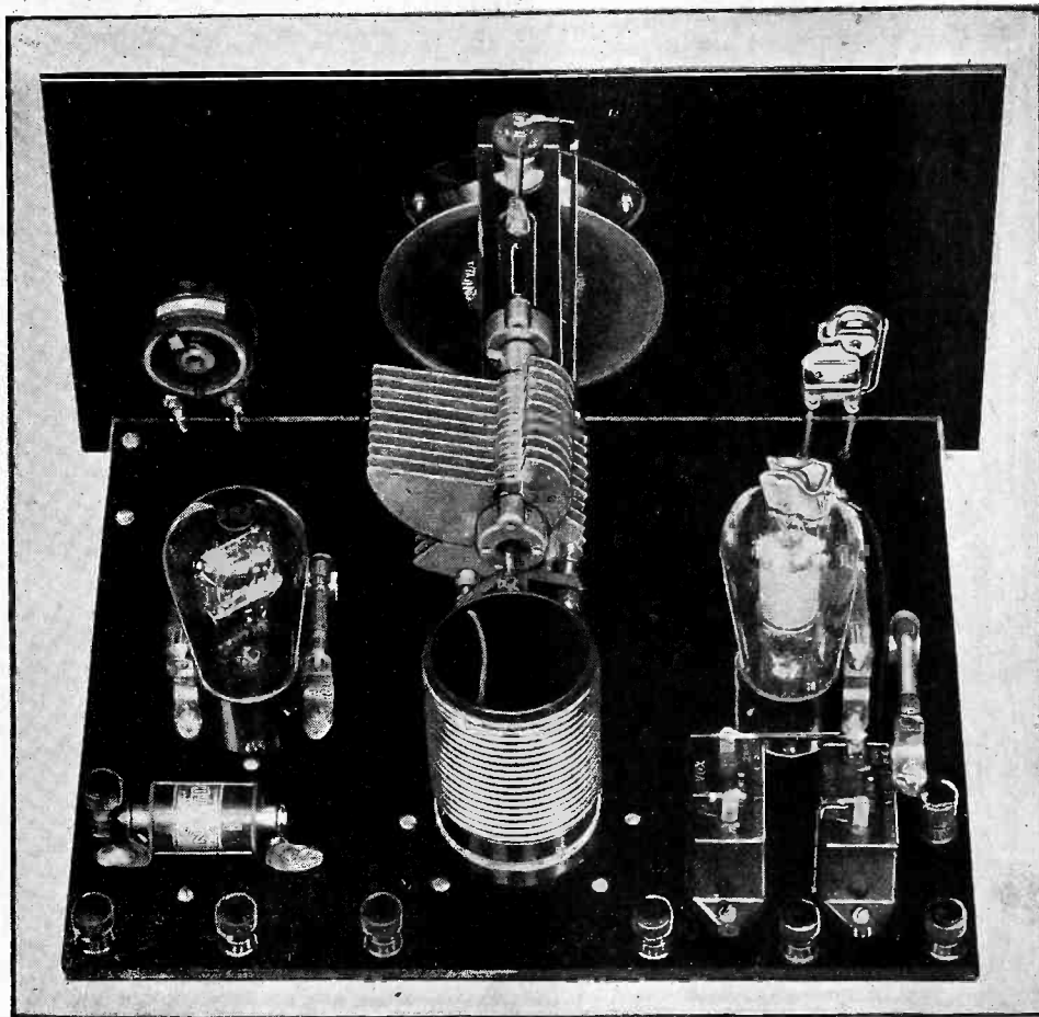
With the National Screen Grid Short-Wave Receiver (above), plus an audio channel, television was received by James Millen. Constructional article begins on page 3. Complete in this issue.
