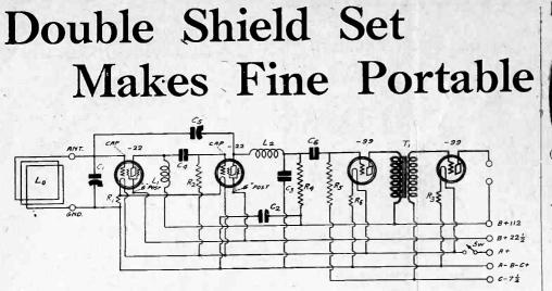
SCHEMATIC DIAGRAM OF THE DOUBLE SHIELD PORTABLE, WITH OP-TIONAL BY-PASS CONDENSERS OMITTED, TO CONFORM PRECISELY TO THE OFFICIAL BLUEPRINT
