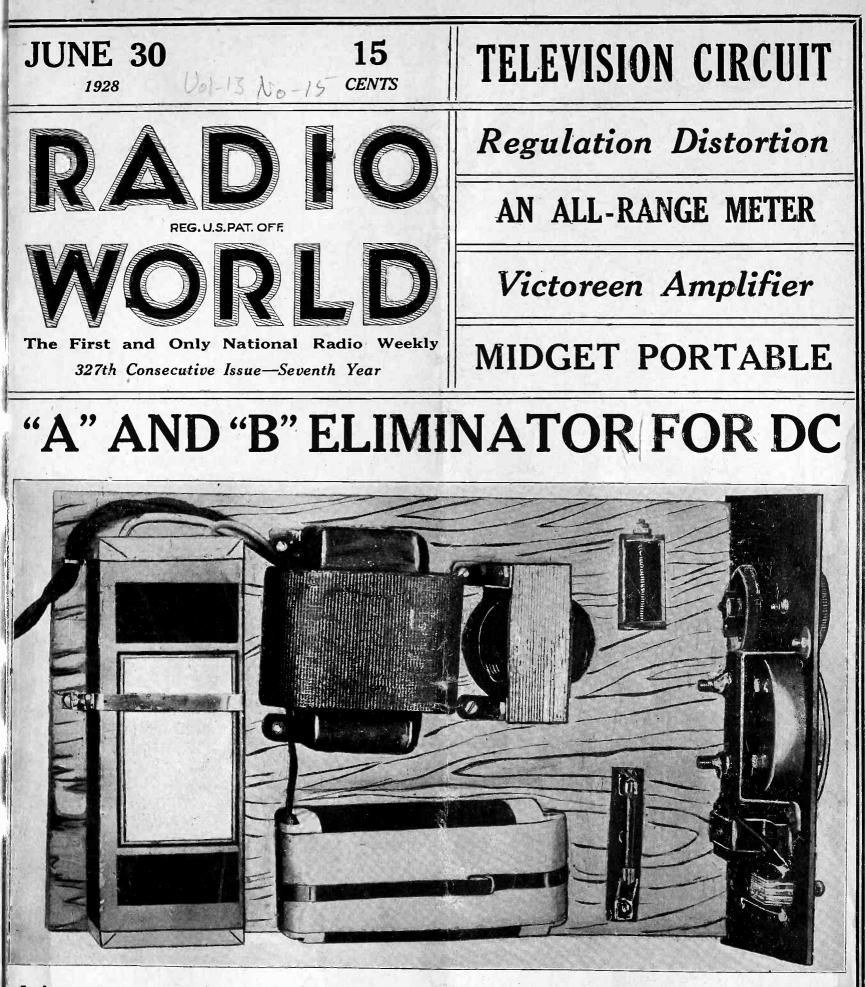
It is very easy to make a DC eliminator for supplying "A" and "B" voltages and currents. View of one is shown above. See page 3.
