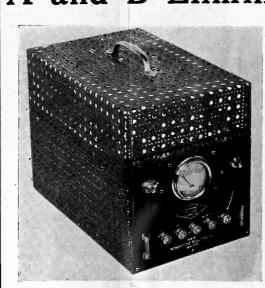
THE COMPLETED DC ELIMINATOR Provides A current and voltage for sets using from 4 to 10 tubes, from the direct current house line, also maximum plate voltage of about 105, with 45 volt tap for detector.
