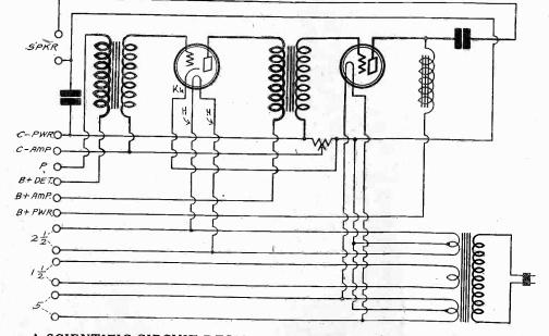
A SCIENTIFIC CIRCUIT DESIGN FOR A TWO-STAGE AC AUDIO AMPLI-FIER, WITH FILAMENT TRANSFORMER AND FILTERED OUTPUT AND BUILT-IN C SUPPLY. THE B VOLTAGES ARE TO BE RECEIVED BY THIS UNIT AND THE FILAMENT VOLTAGES ARE TO BE DELIVERED BY IT TO THE TUNER. THE TUBES USED ARE ONE -26 AND ONE 112 OR -71. NOTE THAT THE MIDTAP OF THE 2½-VOLT WINDING IS MADE POSITIVE IN RESPECT TO THE CATHODE. THIS GREATLY REDUCES HUM.
