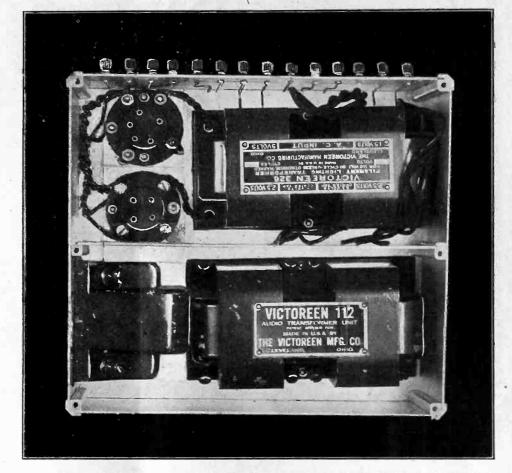
EXACT PLACEMENT OF PARTS PERMITS PARTITIONING THE FILA-MENT TRANSFORMER AND TWO SOCKETS FROM THE TWO-STAGE AUDIO COUPLING AND THE OUTPUT CHOKE (LOWER LEFT). NOTE THAT THE CHOKE IS "HUNG ON THE WALL."
