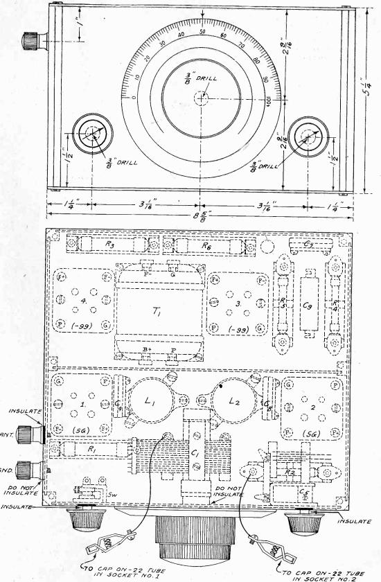
THE FRONT AND THE LAYOUT OF PARTS OF THE DOUBLE SHIELD PORT-ABLE ARE SHOWN HALF-SCALE. THE RECEIVER, CONSISTING OF FOUR TUBES, IS IN ONE SHIELD. ANOTHER SHIELD (NOT SHOWN) CONTAINS THE BATTERIES.
