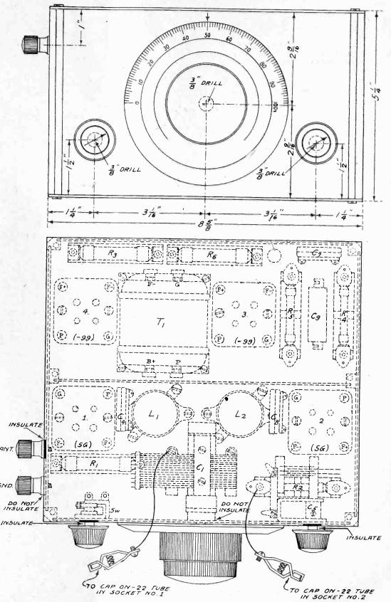
THE FRONT AND THE LAYOUT OF PARTS OF THE DOUBLE SHIELD PORT-ABLE ARE SHOWN HALF-SCALE. THE RECEIVER, CONSISTING OF FOUR TUBES, IS IN ONE SHIELD. ANOTHER SHIELD (NOT SHOWN) CONTAINS THE BATTERIES.
