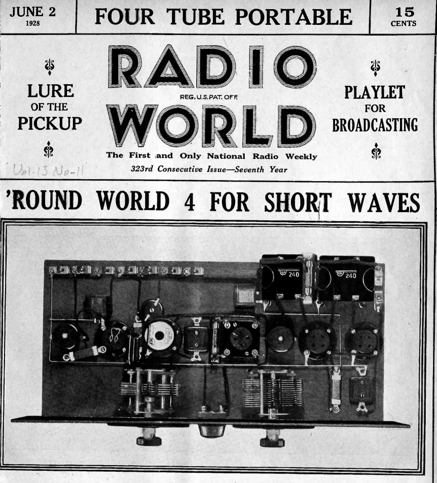
A screen grid RF tube is used ahead of the detector in this brand-new model short-wave set. See page 3.
