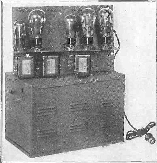
HIGH-POWERED B SUPPLIES, FEEDING INTO LARGE POWER TUBES LIKE THE TYPE —50, ARE BECOMING INCREASINGLY POPULAR. WITH AN UNDISTORTED MAXIMUM POWER OUTPUT OF THE ORDER OF 4,000 MILLIWATTS, WOULD YOU SAY THE POWER TUBE OR THE DETECTOR TUBE WAS THE STRONGER IN THE DISTORTIONLESS REALM?
