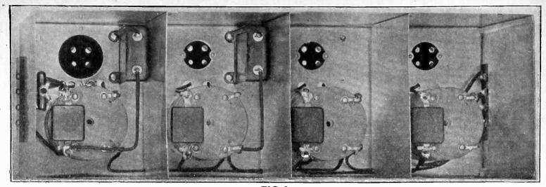
FIG. 2 INTERIOR VIEW OF THE 440 SG INTERMEDIATE FREQUENCY AMPLIFIER USED IN THE SCREEN GRID LAB-ORATORY MODEL SUPER-HETERODYNE. NOTE THE FOUR FIXED FILTER CONDENSER ON TOP OF THE IN-TERMEDIATE COILS, AND THE LARGE BY-PASS CONDENSERS IN THE TWO RIGHT HAND COMPARTMENTS.
