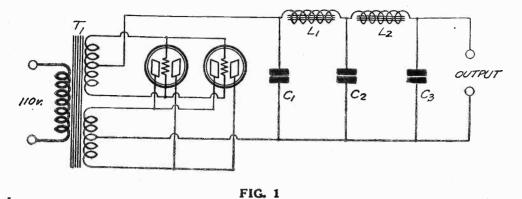
THE CIRCUIT DIAGRAM OF A HEAVY-DUTY B BATTERY ELIMINATOR.
