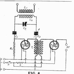
FIG. 6 THE CIRCUIT DIAGRAM OF THE ULTRAUDION TWO RECEIVER DE-SIGNED FOR A BUSY EXECUTIVE AND BASEBALL DEVOTEE.
