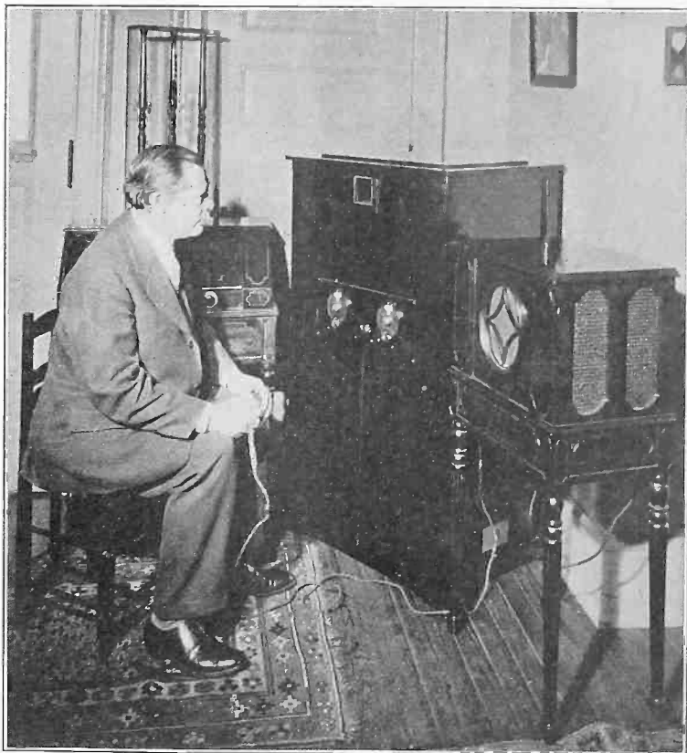
E. F. W. ALEXANDERSON, CHIEF CONSULTING ENGINEER OF THE GENERAL ELECTRIC COMPANY AND INVENTOR OF A SUCCESSFUL TELEVISION APPARATUS FOR HOME USE, SEATED IN FRONT OF A TELEVISION RECEIVER AND VIEWING AN ANIMATED PICTURE SENT BY RADIO FROM THE LABORATORY IN SCHENECTADY. SYNCHRONIZATION BETWEEN THE TRANSMITTER AND THE RECEIVER IS EFFECTED MANUALLY WITH THE LITTLE DEVICE SEEN IN THE HANDS OF THE INVENTOR.
