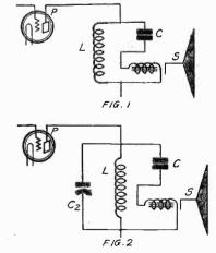
FIG. 1—CIRCUIT DIAGRAM OF AN OUTPUT FILTER AND A LOUD SPEAKER. BOTH THE CONDENSER C AND THE CHOKE COIL L TEND TO SUPPRESS THE LOW TONES. FIG. 2—SIMILAR CIRCUIT WITH A CONDENSER C2 CONNECTED ACROSS THE CHOKE COIL. THIS CONDENSER BY-PASSES THE HIGH FREQUENCIES AND PREVENTS THEIR REPRODUCTION.
