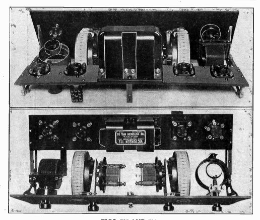
FIGS. 585 AND 586 THE AC300, SHOWING HOW THE PARTS FOR THIS RECEIVER ARE PLACED. THE VICTOREEN 112 AUDIO UNIT IS AT CENTER ON THE SOCKET STRIP.
