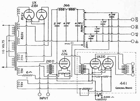
COMPLETE CIRCUIT DIAGRAM OF THE PUSH-PULL AMPLIFIER AND POWER SUPLY DESCRIBED BY MR. WILSON. AN OUTPUT VOLTAGE OF 750 VOLTS DC IS PROVIDED FOR.
