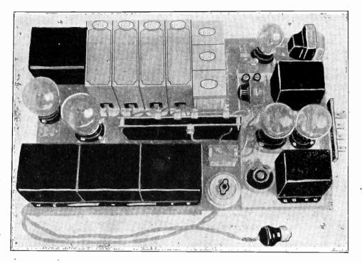
LOOKING AT THE AC UNIT, WITH ITS B SUPPLY AT LEFT AND PUSH-PULL AMPLIFIER AT RIGHT. THE THREE TRANSFORMERS ARE SERIES CONNECTED TO GIVE THE DESIRED HIGH VOLTAGE. THE TOBE CON-DENSERS ARE EXPERTLY PLACED.
