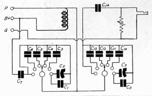
FIG. 3—DIAGRAM OF A CIRCUIT ARRANGEMENT WHEREBY CONDENSERS OF VARIOUS CAPACITIES CAN BE CONNECTED IN SERIES OR IN PAR-ALLEL WITH THE LOUD SPEAKER FOR TESTING THEIR EFFECT ON QUALITY. THE CONSTANTS ARE C1 = .00025 MFD., C2 = .001 MFD. VARI-ABLE; C3 = .0025 MFD.; C4 = .01 MFD.; C5 = .1 MFD.; C6 = .5 MFD.; C7 = 2 MFD.; C8 = .0005 MFD.; C9 = .001 VARIABLE; C10 = .0025 MFD.; C4 = .025 MFD.; C12 = .25 MFD.; C13 = 1 MFD.; C14 = 4 MFD.
