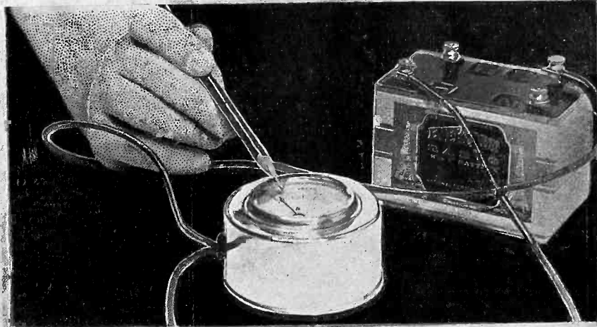
A grid bias battery should be tested with a voltmeter in this manner, never with an ammeter. Only a high resistance voltmeter should be used.
