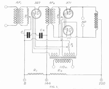
The circuit diagram of a two stage, push-pull power amplifier using one -27 tube and two -71 type tubes. No batteries are used in the circuit.
