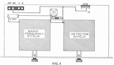
· How the ground connection is made to the shields.
