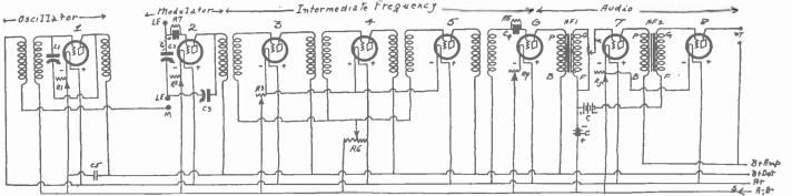
IF a Super-Heterodyne is to be regenerated in the modulator, here's how it's done.
