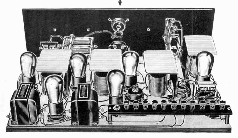
SIX TUBES, All Heated By AC, Are Used IN THIS SET
