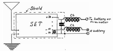
HOW the receiver should be shielded and how choke coils and by-pass condensers should be placed when unshielded batteries or eliminators are used, or when the leads to power source are long.
