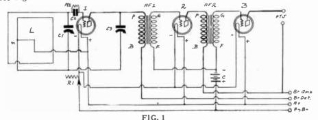
The circuit diagram of a simple three-tube receiver.
