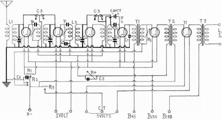
THE PURATONE, A TRANSFORMER COUPLED CIRCUIT in which all the filaments are heated with alternating current. The first five tubes require one volt across the filaments and the last tube requires five volts. The grid bias is obtained through resistance. L2 and L4 are the second and third RFT.
