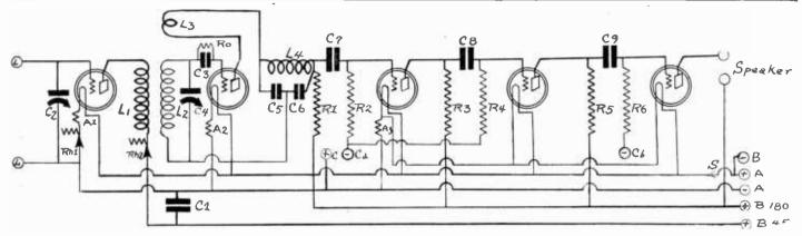
THE circuit diagram of the high quality receiver described by Tim Turkey. Even amplification from the lowest audible to the highest essential frequency is a feature of this receiver. Additional directions for building and operating the receiver are given in the present issue. Freedom from motorboating was emphasized in designing the set.
