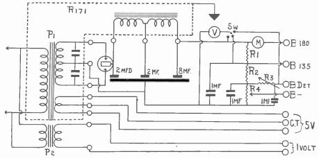
CIRCUIT DIAGRAM of the power supply unit for the six-tube AC heated receiver. The low voltage for the one volt tubes is obtained from a separate step-down transformer P2, the primary of which is connected in parallel with the primary of the power transformer P1.
