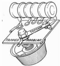
The latest addition to the line of Mount-ford resistances and Kroblaks is the Kro-blak variable resistor of approximately 30,000 ohms, tapped in five equal sections. This unit makes an excellent output control device for B eliminators. The total capacity is 10 watts and the overall size is 2x2x2½ inches. This unit is made by C. E. Mountford, Sullivan Street, New York City.
