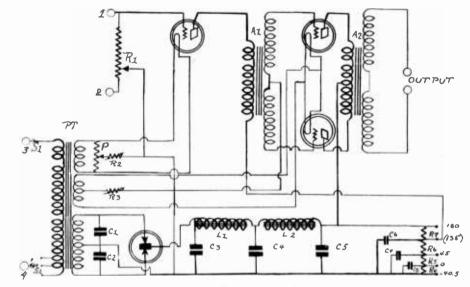
HOW to connect a two stage push-pull power amplifier for amplification of phonograph pick-up and a B battery eliminator. No batteries are used in the device.
