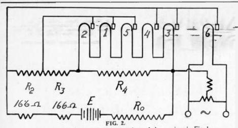
A simplified circuit showing the connections of the receiver in Fig. 1.
