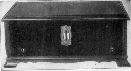
The B. S. T. De Luxe, a 5-Tube Receiver, with Concentrated, Simplified Tuning, and Using Resistance Coupled Audio. Price of set, in genuine walnut cabinet, and including built-in eliminator of all "C" batteries
