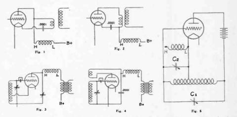
THE radio frequency choke coil is shown in the plate circuit of an RF tube in Figs. 1 and 2, which are equivalent circuits, and in a regenerative detector tube plate circuit, Figs. 3 and 4. The oscillator used for testing the choke coil is Fig. 5.
