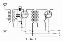
induced in the secondary coil Lg. Lg and C form a combination that may be tuned very closely to the frequency of the incoming signal.
