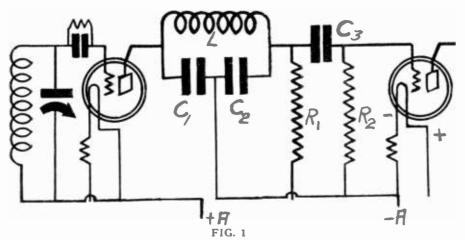
Circuit illustrating the method of connecting the radio frequency choke coil and bypass condensers in the plate circuit of detector in resistance coupled amplifiers for effectively preventing radio frequency currents from entering the amplifier. The same system may be used with other audio circuits. The arrangement is called a low-pass filter.
