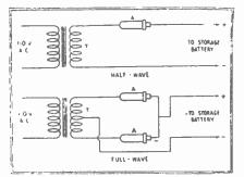
SCHEMATIC diagrams of connections for half-wave and full-wave Raytheon A rectifier. T is the transformer.
