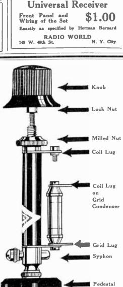
The De Luxe Model Bretwood Variable Grid Leak is shown in actual size. The lock nut secures the knob to the threaded shaft. The milled nut secures the leak to the front panel, if such mounting is desired. The coil lug goes to the outside of the secondary and to the corresponding lug on bullet grid condenser. The grid lug is connected to the grid post of the detector tube socket. The syphon contains the secret resistance element. The pedestal is for baseboard mounting.
