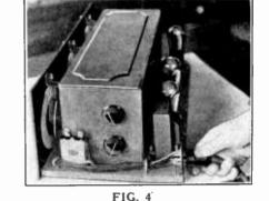
The cable connector leads are distributed by the shortest routes outside the shield to the multiple switch and to points inside the can. Note the placement of the rheostats and the bypass condenser.
