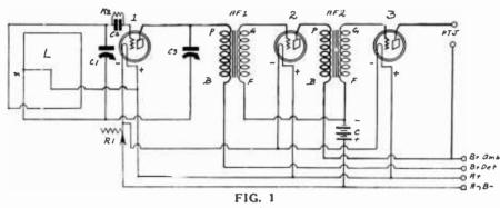
This three-tube set that is operated from a loop runs a speaker in a satisfactory manner and constitutes one of the most economical speaker portables that one can construct.
