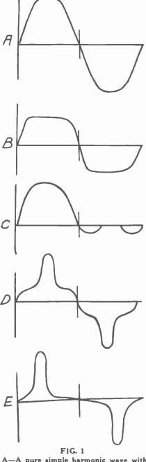
A-A pure simple harmonic wave without higher harmonics. An air wave of a pure tone has this shape.
