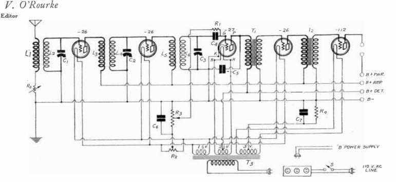
first AF stages. This potentiometer is de-signated by R2 and is an Electrad 20 ohm center tapped fixed resistor.
