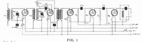
THE DIAMOND OF THE AIR CAN BE CHANGED EASILY SO THAT THE SHORT WAVE STATIONS IN THE BROADCAST BAND WILL BE SPREAD OUT OVER THE ENTIRE DIAL BY CONNECTING THE TUNING CONDENS-ERS ACROSS ONLY A PORTION OF THE TUNING COILS.
