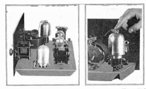
HOW THE RECEIVER LOOKS, AFTER CONSTRUCTION, WITH A VAC-SHIELD ON THE 22 TUBE AND ANOTHER ON THE SPECIAL DETECTOR. ALL THE SPECIFIED PARTS FIT ON THE DRILLED ALUMINUM SUB-PANEL. AT RIGHT, FINGER POINTS TO THE CLIP CONNECTED TO THE CAP OF THE TUBE. THIS CAP PROTRUDES THROUGH THE VAC-SHIELD.
