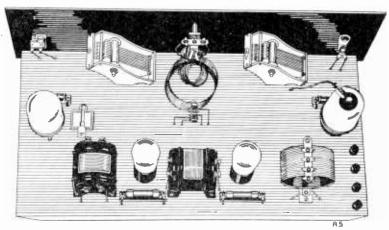
THIS SHOWS THE LAYOUT OF THE PARTS IN THE FOUR TUBE SCREEN GRID DIAMOND. THE BINDING POSTS IN THE LOWER RIGHT CORNER, READING UPWARD, ARE FOR THE PLATE OF THE LAST TUBE AND B+ POWER, RESPEC-TIVELY. THE OTHERS ARE FOR GROUND AND ANTENNA, READING UPWARD.
