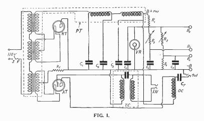
The circuit diagram of the B eliminator and one-stage power amplifier.
