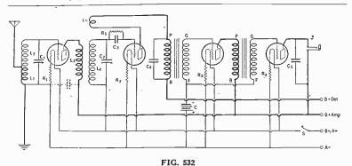
The circuit diagram of the four-tube receiver requested by Frank Merrils.
