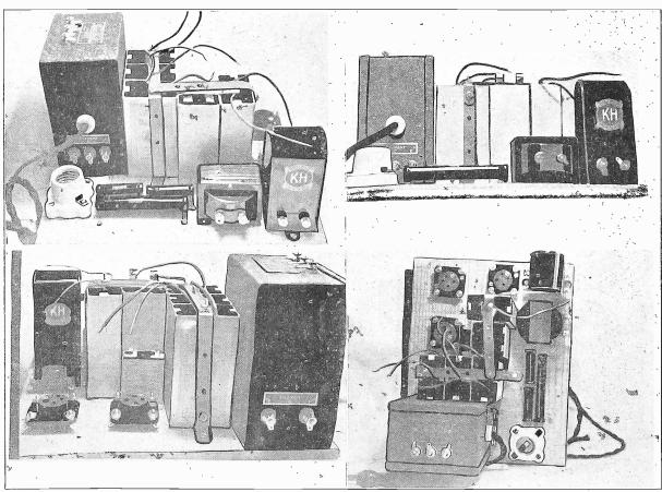
Four general views of the layout of the eliminator. How the Kroblak resistors are mounted is best seen in the photo in the upper left-hand corner. How the sockets are placed to avoid the tubes from hitting each other as well as allowing plenty of play for the insertion of the tubes is shown in the lower left-hand photo. The upper right-hand photo is another view of the resistor mounting. The lower right-hand photo shows exactly how all the parts are placed.
