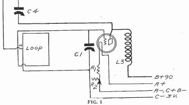
Skeleton diagram showing how to wire the Universal for loop operation.
