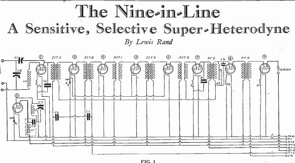
The circuit diagram of the sensitive 9-tube Super-Heterodyne.
