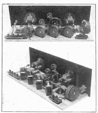
THE baseboard and panel layout of parts is shown in these two photographs. The angular position of the antenna coupler, extreme right, is to be determined experi-mentally. The conventional position is shown, but it is not always the best, as selfoscillation may be strong.
