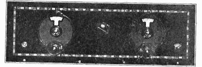
THIS SET has only two tuning controls. Jack, switch and rheostat complete the panel parts.
