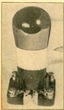
A PIECE of adhesive tape placed between the top of the base and the lowest portion of the glass tube, where the glass is loose in the base, will prevent the tube from moving about, when inserting it in socket. In this way it is possible to prevent the severing of the leads which enter the
