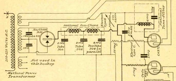
3-Tube AF Channel Has All Plate Voltage Supplied by New B Eliminator, as Well as Filament Heating of Final CX371 and the High Negative Bias for the Grid of That Bulb
