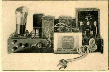
FIG. 6 Rear view of the Lynch Lamp Socket Amplifier.
