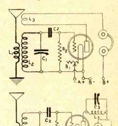
TWO OF the most popular 1-tube circuits that exist today. In the top diagram the rotary tickler coil is used to obtain regeneration, while at the bottom a variable condenser is used with a fixed coil to obtain about the same effect.
