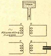
IF DC is applied to condenser plates, the charge is held intact, until saturation point; with AC the charge alternates. Using the tank as an analogy, with DC, the water stores up; with AC, it fills and empties, etc.
