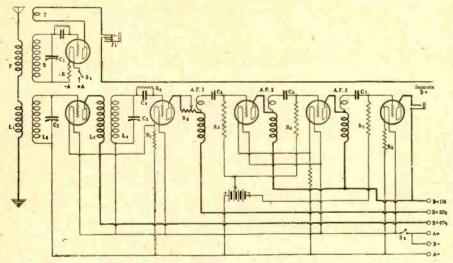
A COMBINATION 1 and 5-tube receiver. The 1-tube receiver may be used for two purposes, as a wavetrap and as an individual receiver. The detectors in both sets are regenerative.
