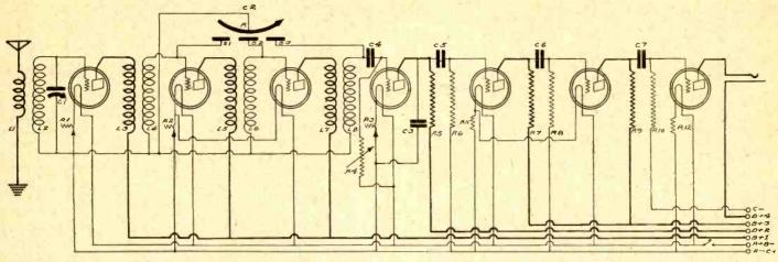
A 7-TUBE receiver, wherein three stages of tuned radio frequency amplification, a non-regenerative detector and three stages of resistance coupled audio frequency amplification are employed. A single condenser is used to tune the secondary of the first or antenna RFT, while the secondaries of the other RFT are tuned by a triple condenser. Standard RFT can be used. The grid return of the detector tube is made to plus A, through the variable grid leak.
