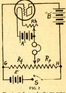
The circuit diagram for the mu-meter.
