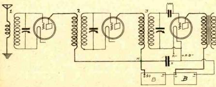
WHERE to connect the by-pass condenser in the radio frequency side of a TRF set is diagrammed above, at point X. M indicates the common B voltage terminal for the RF amplifier tubes.
